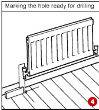
There are two ways to run pipes - from beneath the floor or along the surface of a wall. If the pipes are coming from beneath a wooden floor, you need to mark and drill holes (4). The best way to do this is with a right angle of some kind. Hold a try square in line with the centre of the valve in two positions and mark the points on the floor. Where the lines cross on the floor
