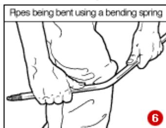
Pipes can be bent by inserting a bending spring of the correct size and gently bending the pipe over a rounded object. Slightly over-bend past the angle and then bend back to release the spring (6).
